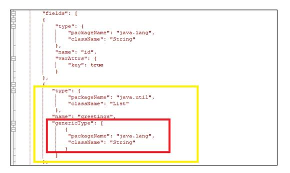
Within the "type" of the field provide a generic type JSON array where each element of the array provides the package name and the class name of the parameterized types. In the example above the parameterized type is a String class of Java.
